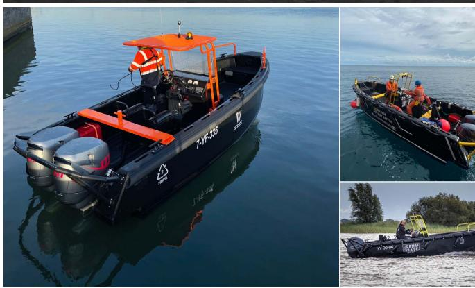
The RBB 700 is our smallest and most versatile platform. Our customers use this 7 metre workboat for dive support, surveying, patrolling and crew tendering. The unsinkable HDPE hull has a flexible layout to accommodate all your requirements: dive door, push bow, towing bit etc. The boat can be equipped with all modern navigation and communication equipment. Propulsion by gasoline or diesel outboards or diesel waterjet.
