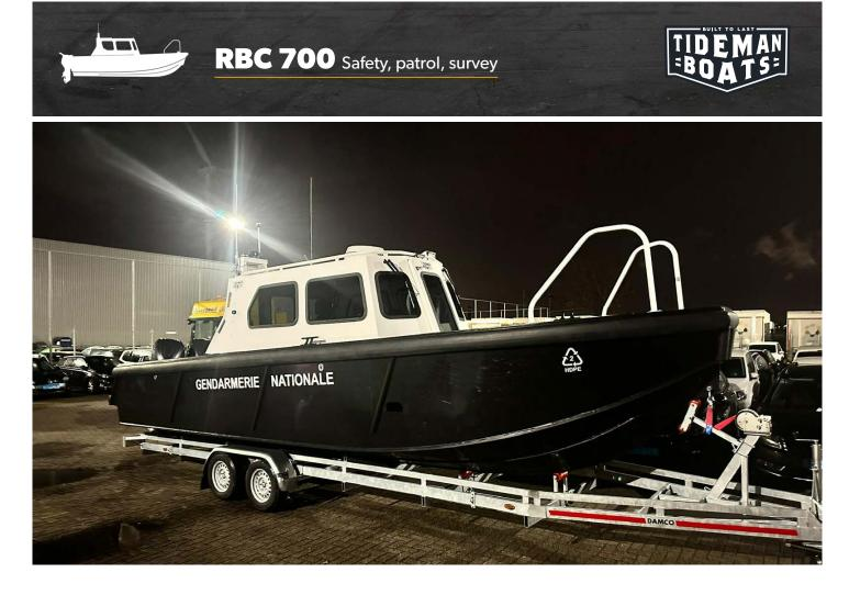
The RBC 700 is our smallest and most versatile cabin workboat. Our customers use this 7 metre workboat for dive support, surveying, patrolling and crew tendering. The unsinkable HDPE hull has a flexible layout to accommodate all your requirements: dive door, push bow, towing bit etc. The boat can be equipped with all modern navigation and communication equipment and is fully trailerable.
