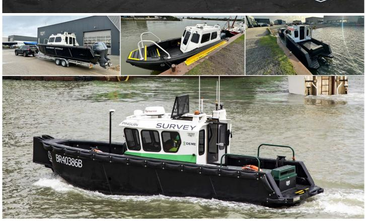
The RBC 900 is our midsize cabin workboat. Our customers use this 9 metre workboat for dive support, surveying, patrolling and crew tendering. The unsinkable HDPE hull has a flexible layout to accommodate all your requirements: dive door, push bow, towing bit etc. The boat can be equipped with all modern navigation and communication equipment and is fully trailerable.
