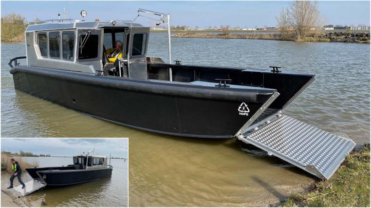
The LCC 1000 is our cabin landing craft. Our customers use this 10-metre workboat to transport people and supplies from ship to shore. The unsinkable HDPE hull has a flexible layout to accommodate all your requirements: dive door, towing bit etc. The boat can be equipped with all modern navigation and communication equipment and is fully trailerable.
